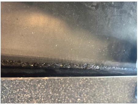
Figure 1. Debris from dumbbells seen in cracks of rack. This debris is caused by the edge of the rack clipping the rubber on the dumbbells.
