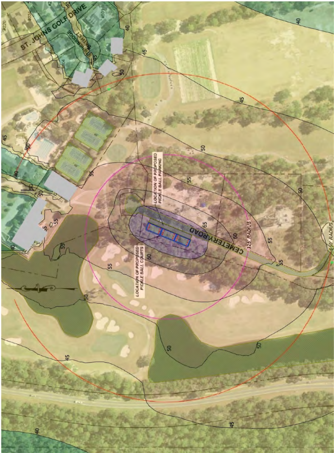
Figure 3.3. Adjusted Sound Pressure Level Contours for Proposed Pickleball Courts
